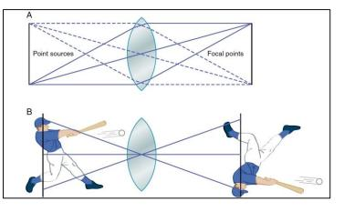
When light rays traveling through a transparent substance pass into a second transparent substance with a different density, they bend at the junction between the two substances (**refraction**).
