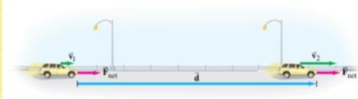
FIGURE 6-7 A constant net force  $F_{\text{net}}$  accelerates a car from speed  $v_i$  to speed  $v_f$  over a displacement  $d$ . The net work done is  $W_{\text{net}} = F_{\text{net}}d$ .
